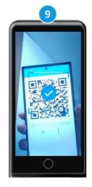
During this step you can see your QR code position on the inner lock display to adjust QR code in the given marking positions
